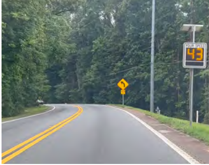
Speed Limit Detection Signage Along a Tight Horizontal Curve on Browns Mill Rd Between E Saddle Ridge Dr and Evans Mill Rd
